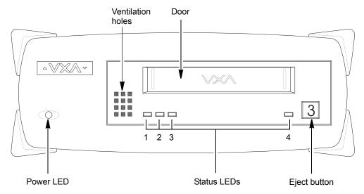
Figure 1-3 External tape drive: front-panel components
